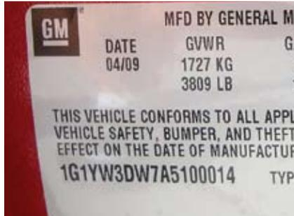
Digit 8 is still the engine code: "W" is the 6.2L LS3, "E" is the 7.0 LS7 and "T" is the 6.2L Supercharged LS9.
